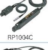
RP1004C | Current Probe                    | BW: DC to 100 MHz<br>Max. input<br>AC P-P: 50 A (noncontinuous),<br>AC RMS: 30 A<br>Compatibility: all <b>RIGOL</b> scopes.<br>Must order RP1000P power supply.                                      |
