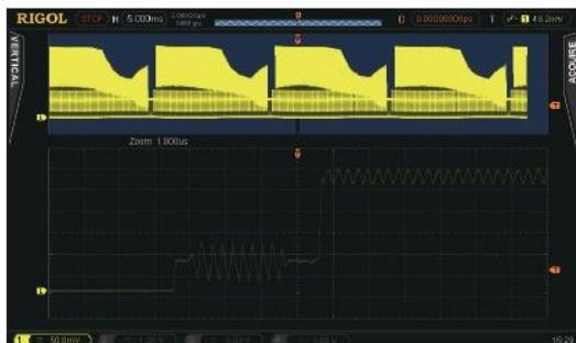
Provide the capability to see both the panorama and detail simultaneously
