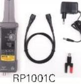
RP1001C   | Current Probe                    | BW: DC to 300 kHz<br>Max. input<br>DC: $\pm 100$ A,<br>AC P-P: 200 A,<br>AC RMS: 70 A<br>Compatibility: all <b>RIGOL</b> scopes.                                                                     |
