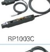
RP1003C  | Current Probe                    | BW: DC to 50 MHz<br>Max. input<br>AC P-P: 50 A (noncontinuous),<br>AC RMS: 30 A<br>Compatibility: all <b>RIGOL</b> scopes.<br>Must order RP1000P power supply.                                       |
